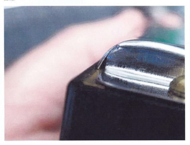
However, with the increased heights of both the blow and draw reed plates, the leading edge of the cover plates will now sit "on-top." I originally thought this would be a problem regarding air leakage, but was pleased to discover it was a non-issue.
