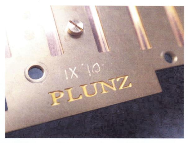
For harmonica players not familiar with the concept of thicker reed plates, it is a design strategy that is intended to provide the reeds with *more power*. This is accomplished by enabling the existing (stock) harmonica reeds to swing further down into the chamber (slot). More air passes across the reed increasing volume and response. As always, proper offsetting (gapping) is essential to maximize the benefits—Bernoulli Effect anyone?
